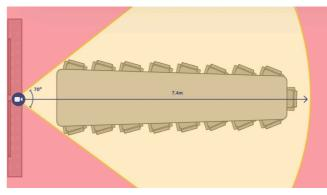
Rooms that are greater than 4m should be equipped with a camera that has optical zoom and a narrower field of view. This optimises the ability for the camera to pick up in-room participants at a distance. Functions such as speaker tracking or intelligent framing options allow for a richer remote experience.
